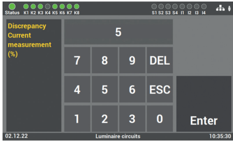
Fig. 91: "Threshold values" mask (electrical circuit monitoring)
